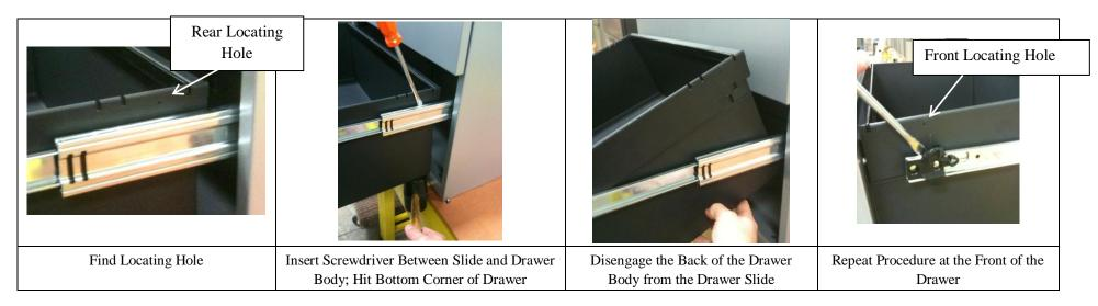
To reinstall the drawer, align the attachment holes on each side of the drawer body with the corresponding tabs on the drawer slide. Slide the tabs into the holes on the drawer body. Make sure that the drawer is firmly pushed down and secured to the slides.
